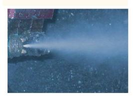
**DILUCO<sup>™</sup> 1041** is a high performance, water-based lubricant developed for use in aluminum and magnesium die casting applications. Formulated for medium to large, functional and automotive parts; the product provides, high quality castings with exceptional cosmetics and will not interfere with painting or plating. The chemically balanced blend of natural lubricants, unique polymers and wetting additives provide excellent finish and metal flow without in-cavity or over-spray build-up.
