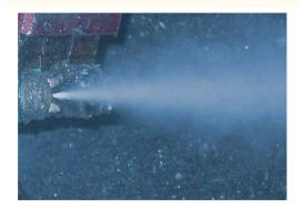
**DILUCO™ SU-2650 G** is a high performance, polymer-based release agent to be used during the initial startup phase of the die casting process. Its blend of natural lubricants along with dispersed graphite helps prevent sticking during the first few shots of startup. It also assists with the lubrication of the ejector pins, slides, fins, and core areas.
